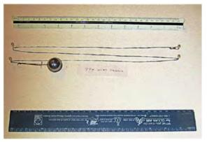
Figure 1. 994 mm Test Pendulum
